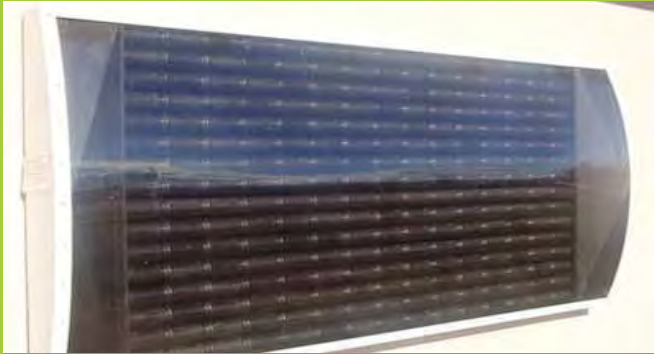
A solar to air collector, constructed with recycled cans, provides heat on sunny days.
