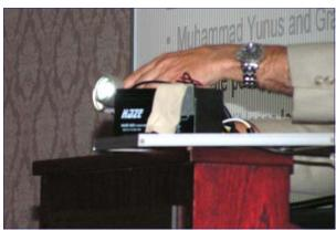
Above: The small yet powerful light developed for the Light Up The World project. It is powered by a special battery pack that lasts for four years and is recharged by either an 8 x 11-inch solar panel or a pedal charger. The unit costs just \$200 and is already in over 16,000 homes around the world.
